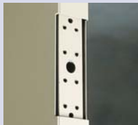
Standard Non-handed hinge preparation. (minimum 10 gauge). Prepare for standard and heavy weight 4.5" Hinges
